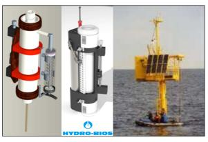
**Figure 14:** On the left side the "old" AFIS sampler is depicted. This sampler was used during the AL439 cruise (left). The next graph shows the Prototype of the newly developed AFIS sampler, which will be used for upcoming sampling opportunities (middle). The graph on the right side represents the fixed Marnet station Darßer Schwelle (right).
