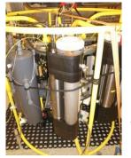
Figure 18: CTD with regular free-flow bottles (left) and new AFIS (right). Photo: C. Bennke
