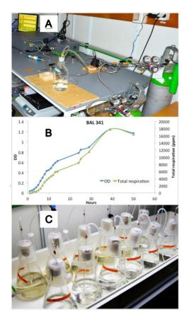
**Figure 8**: Technical setup for the Picarro  $\delta$ 13C carbon dioxide analyzer (A). Growth performance results for heterotrophic Baltic Sea model bacteria using Picarro (B). Model bacteria growing in organic matter from different phytoplankton species (C).
